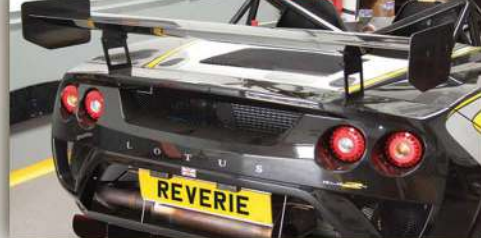
3 300MM HIGH DOWNFORCE WING ON LOTUS 2-ELEVEN
