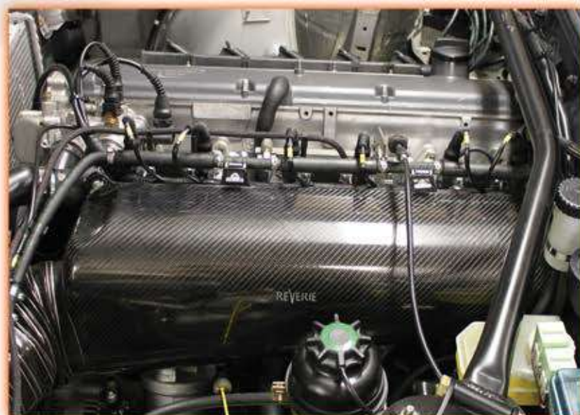
BMW E30 M30 courtesy of Erik Tryggvesson Fitted with LH Zolder 6 Cyl Airbox
