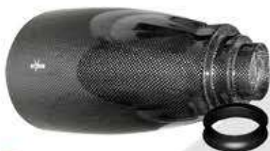
Daytona 230 carbon fibre canister, 152mm inlet, 100 / 75 / 58mm outlet for use with bespoke to Reverie cone filter. Filter flows 166 cfm at 1.5" H 2 O using 100mm inlet/outlet
