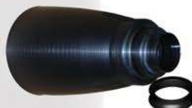
Daytona 230 TT filter canister, shorter than standard Daytona 152mm inlet, 100 / 75 / 58mm outlet for use with Reverie cone filter. Filter flows 166 cfm at 1.5" H 2 O using 100mm inlet/outlet
