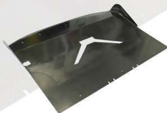
Caterham diffuser for De-Dion axle available as SV wide or Non SV versions Centre cut out shown on diffuser (above image) is not required for cars with newer independent rear suspension
