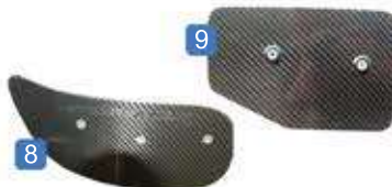
Carbon fibre wing endplates 8 Standed Noble m400 style R01SB0348 9 Rectangular 2-Eleven style R01SB0356
