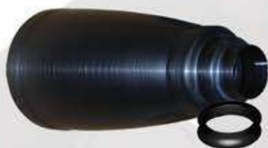
Daytona 230 alloy canister, 152mm inlet, 100 / 75 / 58mm outlet for use with bespoke to Reverie cone filter. Filter flows 166 cfm at 1.5" H 2 O using 100mm inlet/outlet
